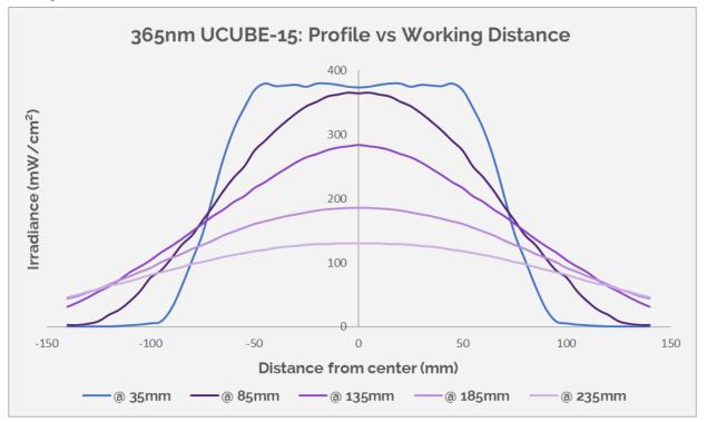
Curve plotted for UVA wavelength. For UVC & UVB irradiance, please divide the irradiance value by a factor of 40. Radiometer: GIGA HERTZ OPTIK RCH-116 (June 2023). For the UV spot graph, the spot size is the exposed area where the irradiance is higher than 50% of the maximum irradiance.
