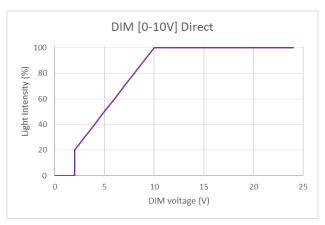
Other Dimming signals are available upon request: 0-24V indirect, 0-10V direct, 0-10V indirect, 0-5V direct or 0-5V indirect.
